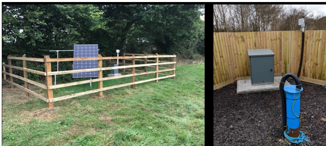
Figure 3: Photographs of two UDDGP microseismic stations. A) a broad-band seismometer station powered by 12V deep-cycle batteries, with continuous recharging via solar-panels. B) a borehole geophone station using mains power and backup batteries. The wellhead standpipe is blue and the black conduit carries the geophone cable underground into the instrumentation cabinet.
