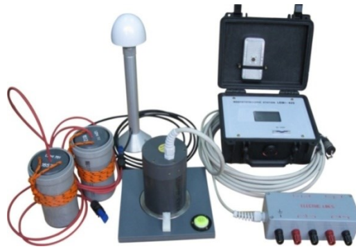
Figure 1: General view of the LEMI-424 magnetotelluric station.
