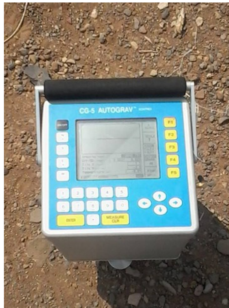
Figure 8 : A : Scintrex CG5 Gravimeter, B : Field photo during an Gravity survey.
