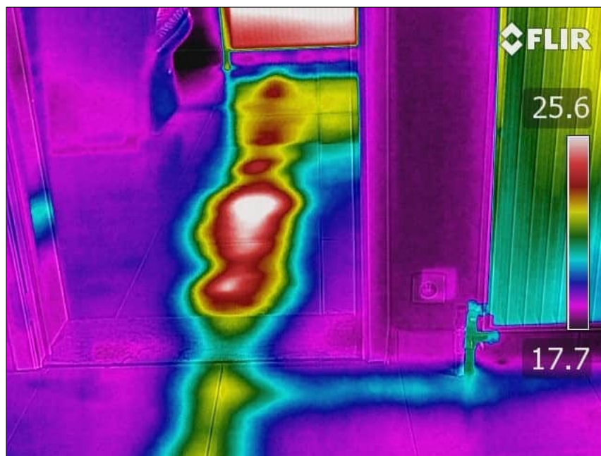
Figure 1: A heat source detected beneath a solid floor by a thermal infrared camera. Heat conducts through the floor to the surface, from where it radiates and convects into the air. Directly mapping the conductive heat flux through the surface of the floor could fully constrain the location, depth and magnitude of the heat source. Source: https://www.cibor.be/en/cibor-scores-infrared-leak-detection-camera-inspection-piping/
