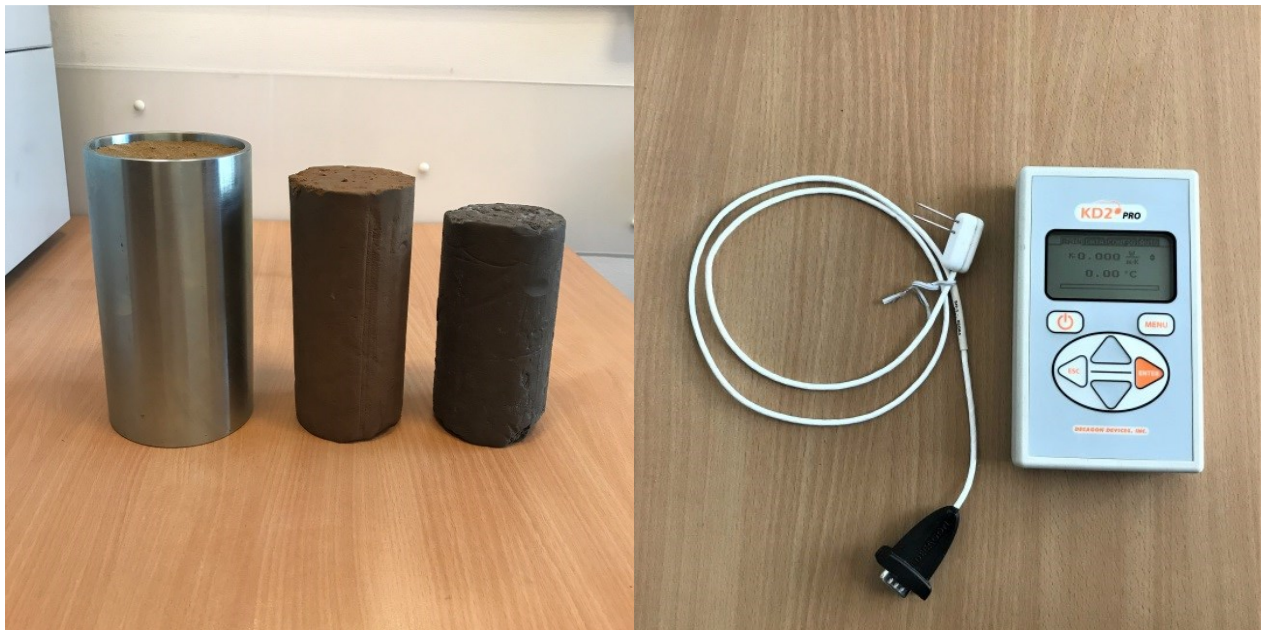
Figure 1. Left: Analyzed samples after three cycles of freezing and thawing (medium sand, silt, clay), right: KD2Pro Thermal Properties Analyzer with SH-1 dual needle sensor.
