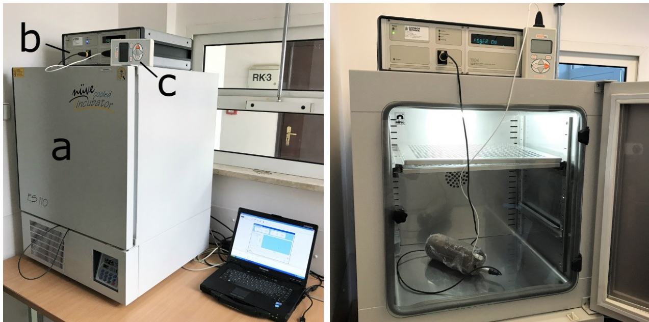
Figure 2 Left: measuring equipment: a. laboratory incubator, b. TK04 measuring unit, c. KD2 Pro Thermal Properties Analyzer, right: undisturbed cohesive soil sample during measurements.
