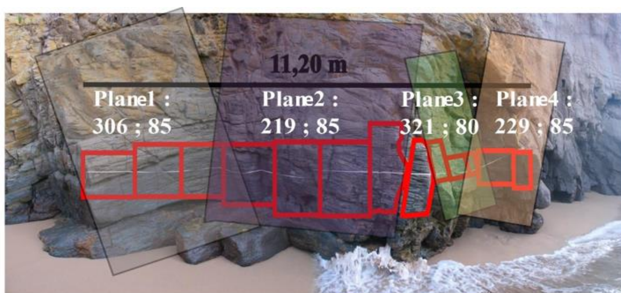
Figure 5: Photograph of the outcrop at Tillet Creek along the first 11.2m of the scanline. Each red shape represents a picture in which fractures were digitized. They belong to fracture planes (plane 1 to 4) which orientation, expressed as “dip direction; dip” (e.g. 306; 85 for plane 1), gives the outcrop its particular geometry.
