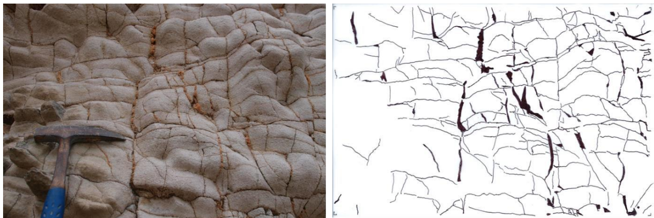
Figure 9: Example of surface occupied by filling or aperture of discontinuities (7.6%) and intensity of these discontinuities (P21=0.24cm/cm 2 ).
