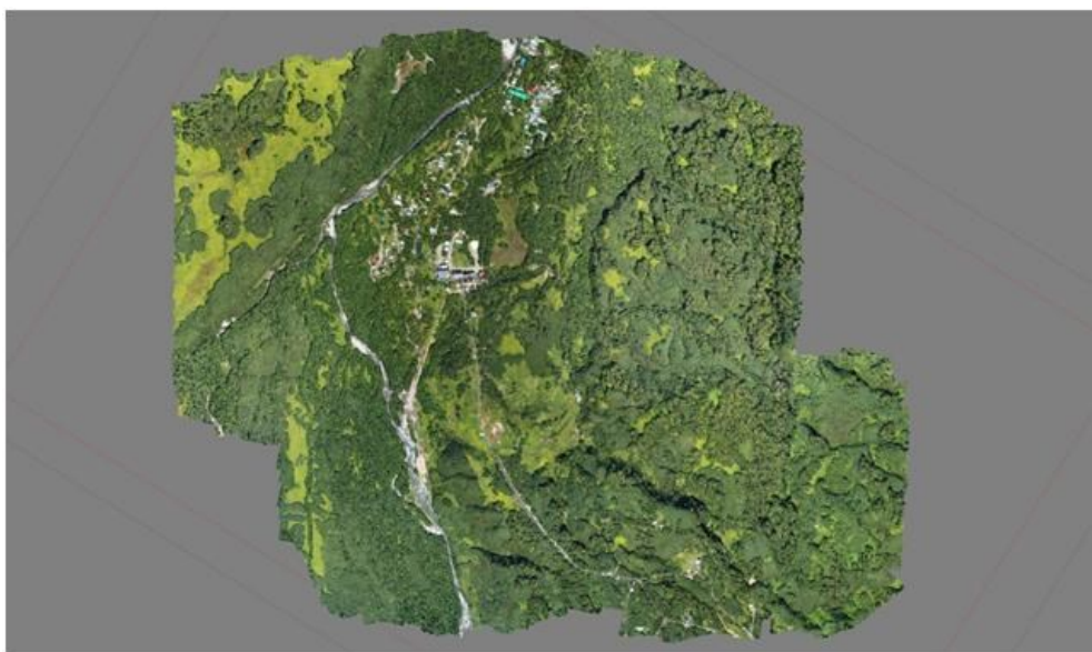
Figure 2: Dense point cloud. Project of 3000 photos of the Pauhetsky hydrothermal deposit area.
