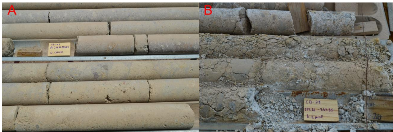
Figure 4: Here we show two examples from the PGC-01 well. Image (A) represents the consolidated samples which are most common along the well, while (B) is an example of the unconsolidated samples found in specific zones.
