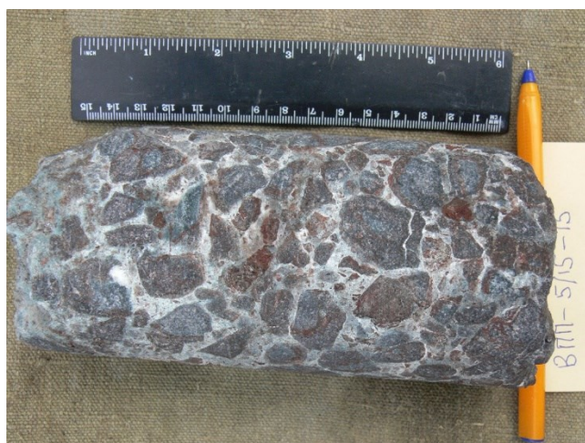
Figure 4: Andesitic metasomatic breccia (sample VPP-5/15-15)
