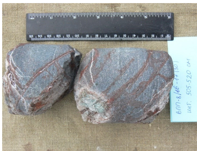
Figure 5: Slightly altered fractured andesite (sample VPP-8/16-17)
