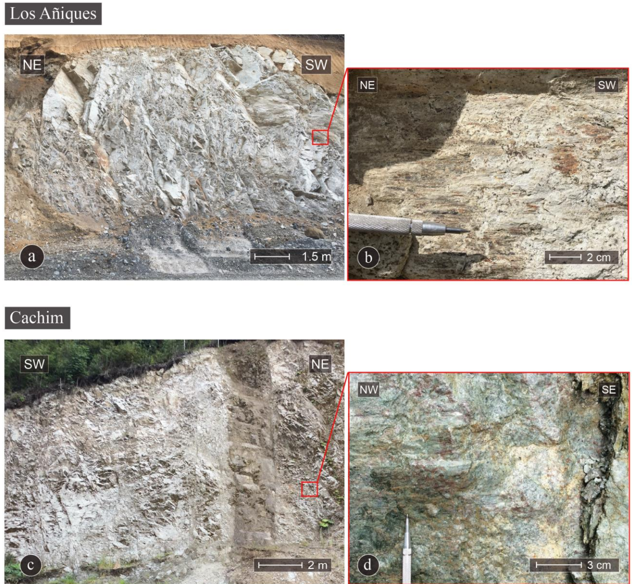
Figure 3: Structural sites chosen for this study. a) Los Añiques structural site is related to LOFS exposure (strike of regional fault N30°E). b) Example of fault in Los Añiques structural site; c) Cachim structural site is related to ATF exposure (strike of regional fault N70°W). d) Example of fault in Cachim structural site.
