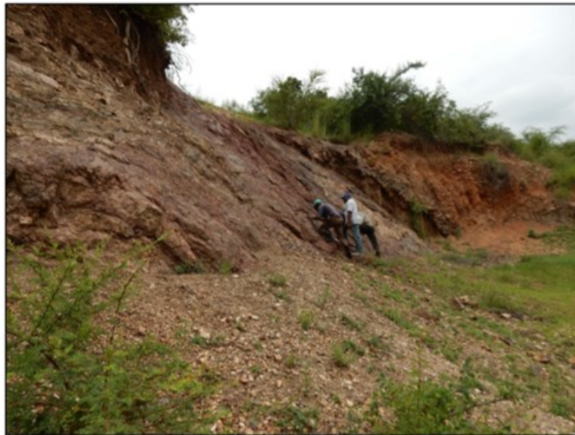
Figure 4: MEMD staff Edward Isabirye, James Natukunda, and Isa Lugaizi, collecting structural data on a fault surface associated with the Lower fault, locally dipping 43° E.
