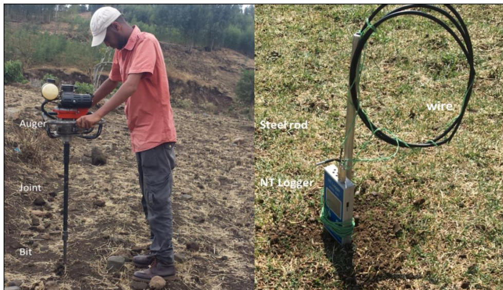
Figure 5. Tools used during soil temperature measurements.
