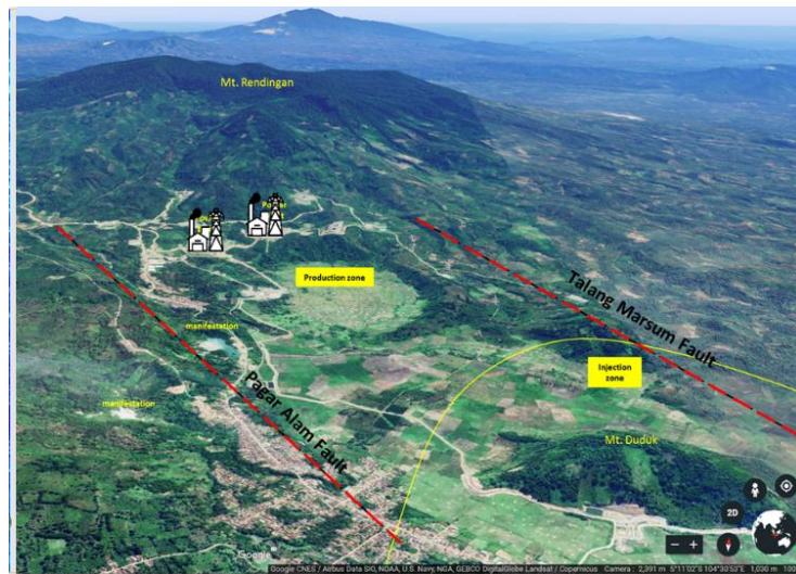
Figure 1: The figure of Ulubelu geothermal field from surface model and satellite image taken in early 2019 showing the distribution of structures, manifestations, production - injection zone, and power plants location.
