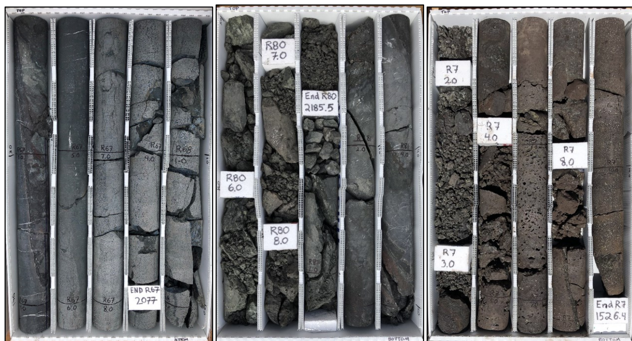
Figure 9: Cleaned, cut, and boxed rock core recovered from the deepened Lānaʻi Well 10. (Left) Example of solid, consolidated units within the borehole. Evidence of a high-angle dike intrusion into the surrounding rock (left-most column in the core box). (Center, Right) Example of friable formations downhole. Most of this material came out of the core tube in a fairly competent form but clearly broke apart as they dried. This was milled up in between the drill string and the borehole walls into a fine sand.
