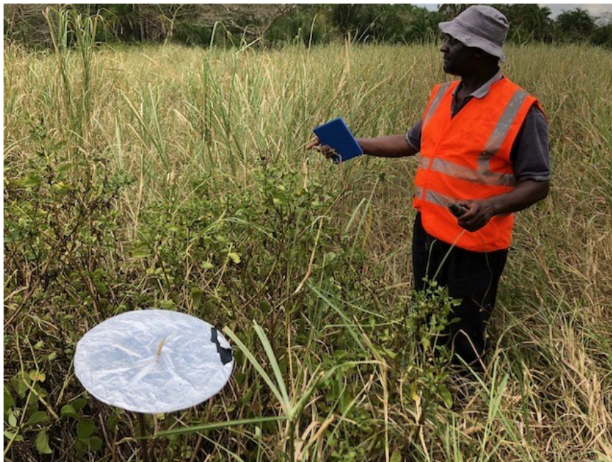
Figure 5: GCP made from a 12" vinyl record covered with aluminium foil.
