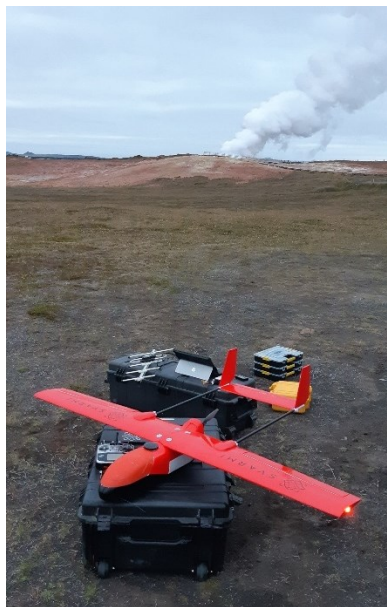
Figure 2. The fixed-wing UAV equipped with a thermal sensor used by Svarmi ehf to create thermal datasets at Reykjanes geothermal area in summer 2018.
