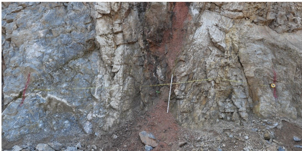
Figure 2: Exemplary scanline setup in the quarry Hagen-Hohenlimburg intersecting different facies types.
