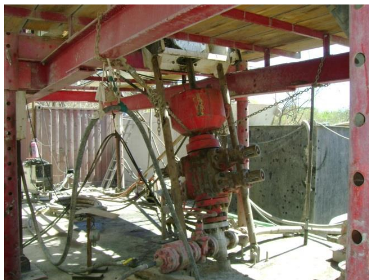
Figure 6: Blowout Preventer for slanted slimhole drilling.
