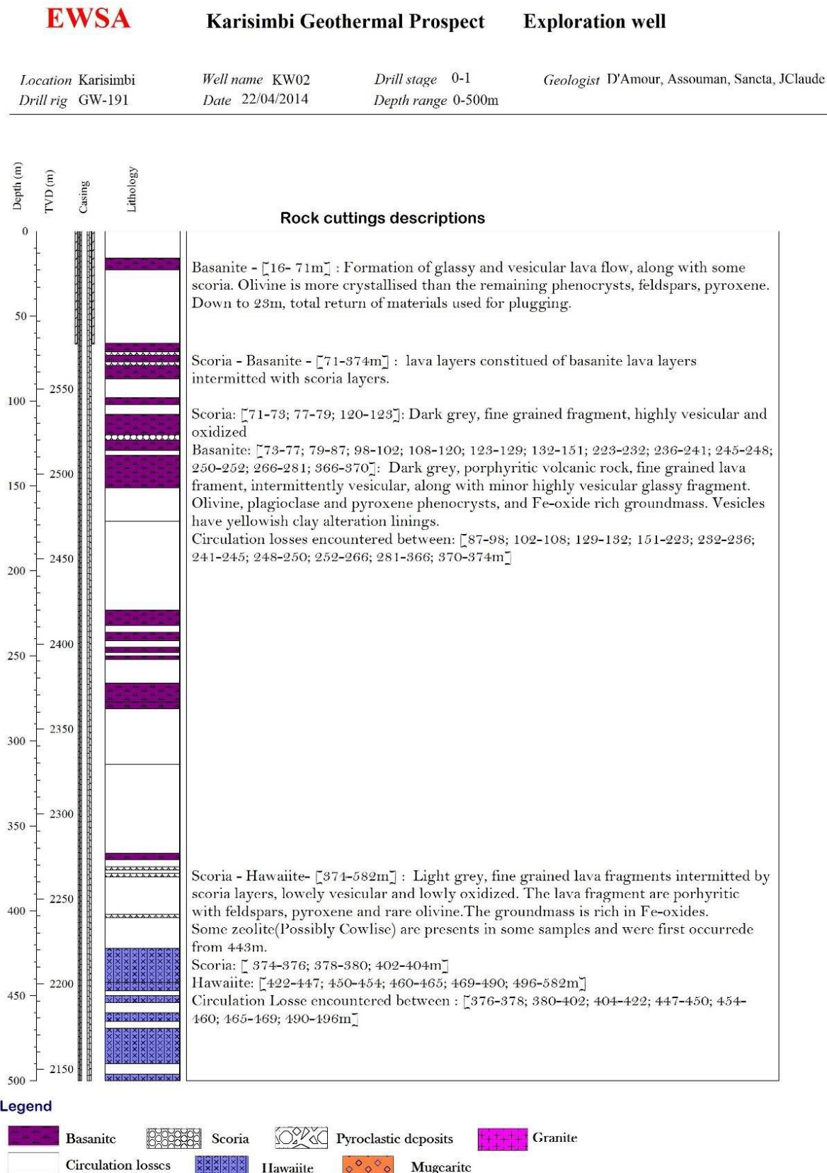
Figure 11: Stratigraphic log of well KW02 from 0 to 500m.
