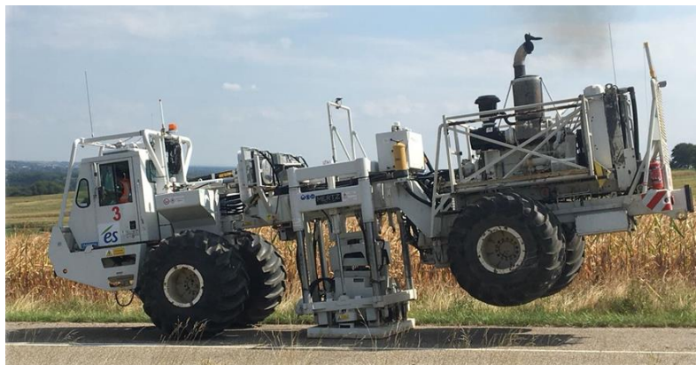
Figure 8: Mertz 26HD-623B (deployed number: 9) - Peak force output 276 kN (62 000 lb). One AHV- Peak force output 275 kN (62 000 lb) with soundproofing system was also deployed but mainly in cities. (Source ESG)
