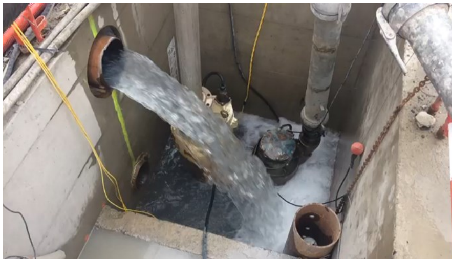
Figure 12: Artesian water flow from Géo-01 at 34°C and 50 l/s
