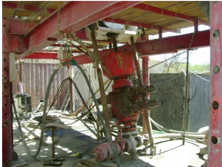
Figure 5: Typical slimhole coring rig. Figure 6: Blowout Preventer for slanted slimhole drilling.
