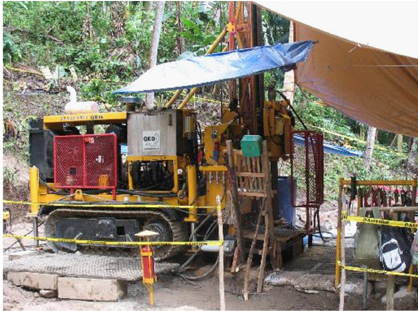
Figure 8: A small coring rig drilling with HQ to depths of 1250 m into temperatures beyond 200°C.
