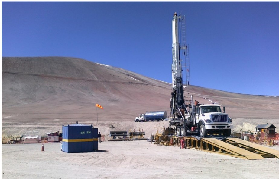
Figure 6: A ~ 20 ton hook load, truck mounted coring drillrig drilling a hybrid well in Chile.
