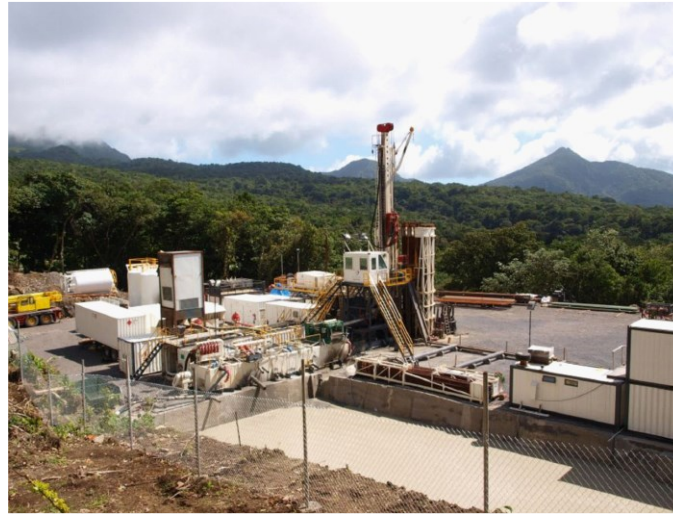
Figure 4: A 100 ton hook load drillrig (Sleipnir, Iceland Drilling), drilling a well with 6 1/8" open hole section in Dominica. Three wells were drilled to 1600-1800 meters.
