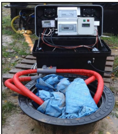
Figure 8: Thermal Response Test device while measurements
