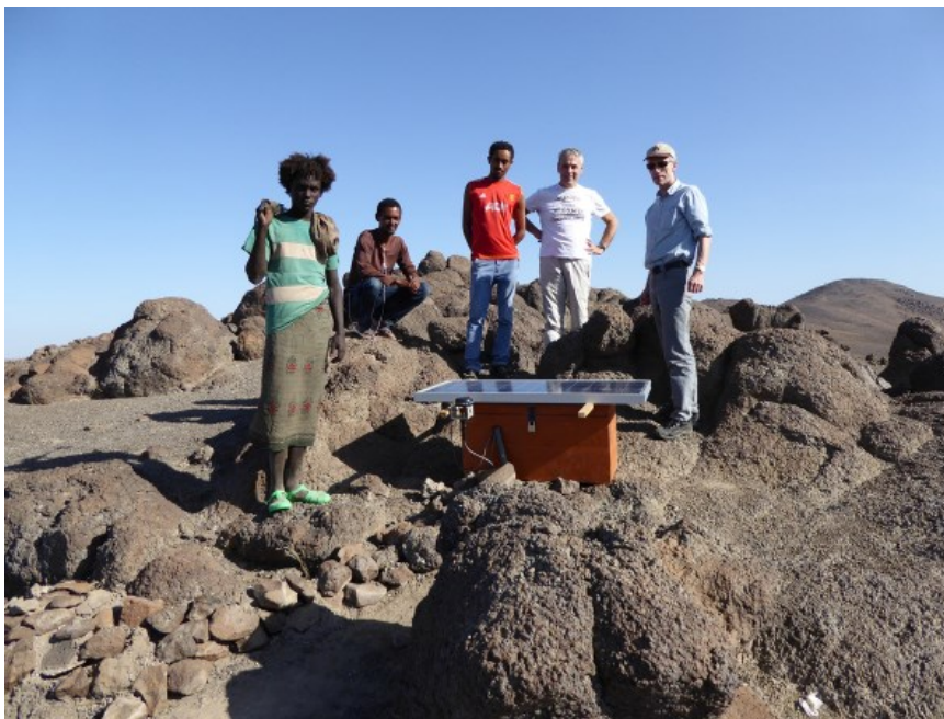
Figure 2. Setting up an MT station at Lake Abhé in Djibouti for resistivity surveying.
