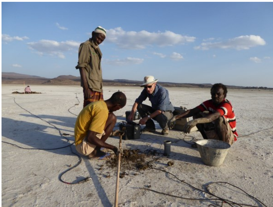
Figure 2. Setting up an MT station at Lake Abhé in Djibouti for resistivity surveying.
