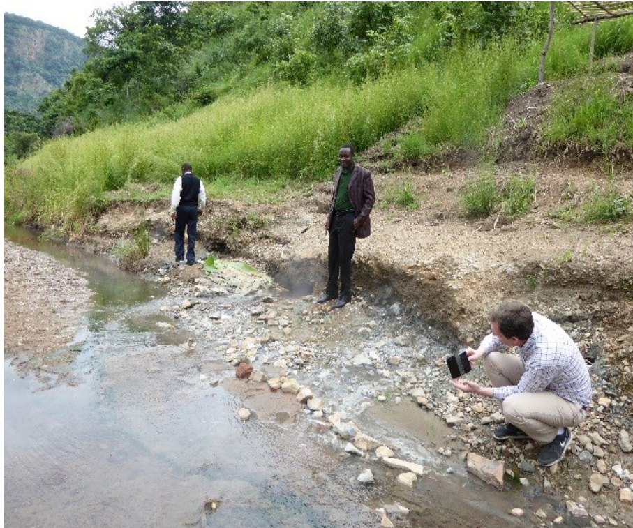
Figure 5. Exploring geothermal in Chiweta, Malawi – geothermal fluid flow (80°C) is connected to a fracture, smell of sulfur and yellow sulfur alteration is seen on the surface.
