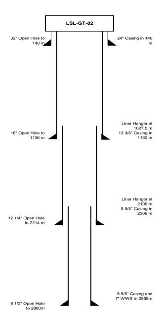
Figure 3: Well schematic of LSL-GT-02.
