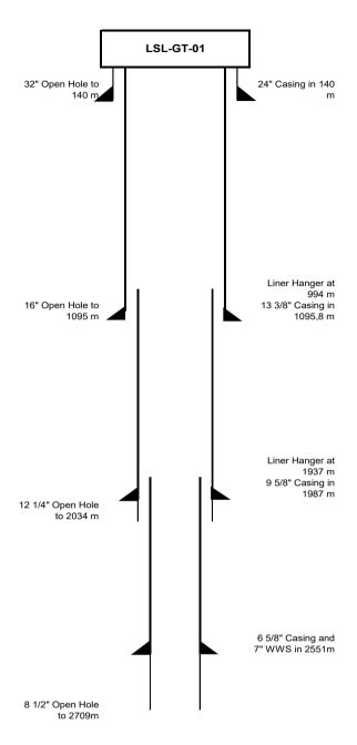
Figure 2: Well schematic of LSL-GT-01.
