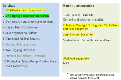
The drilling rig and equipment (marked green) only represents around 40-45% of the total drilling cost. It is highly misleading to compare day rates in different countries having different contract cultures, as some of the services or equipment may be charged separately and outside of the traditional day rate. Lower rig day rate does not necessary at the end represent higher or lower total cost.
