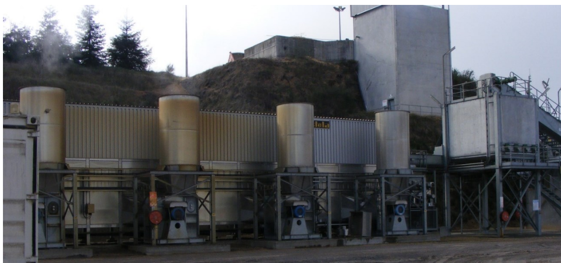
Figure 6: Nature's Flame Wood Shaving and Sawdust Belt Drier(s) converting to geothermal energy. Photo credit: Brian Carey, GNS Science.
