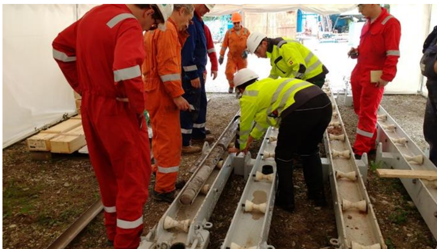
Figure 3: Retrieval of the drilling cores in aluminium half-shell liners, sawn to 1 m pieces.
