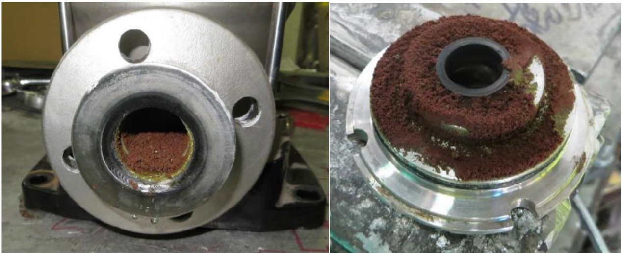
Figure 3: Selenium deposits in condensate pumps of the gas removal system.
