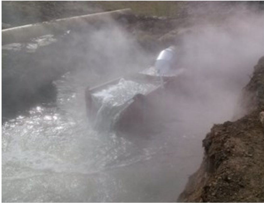
Figure 8. V-formed weir box for flow measure. The flow from the well with an air-lift from 323 m about exceeds the flow capacity of the weir-box and was estimated at least 125 l/s.
