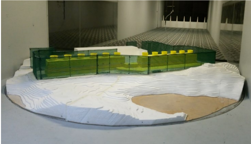
Figure 10: Wind Tunnel Model of Bacman-Palayan Cooling Tower with Wind Fence.
