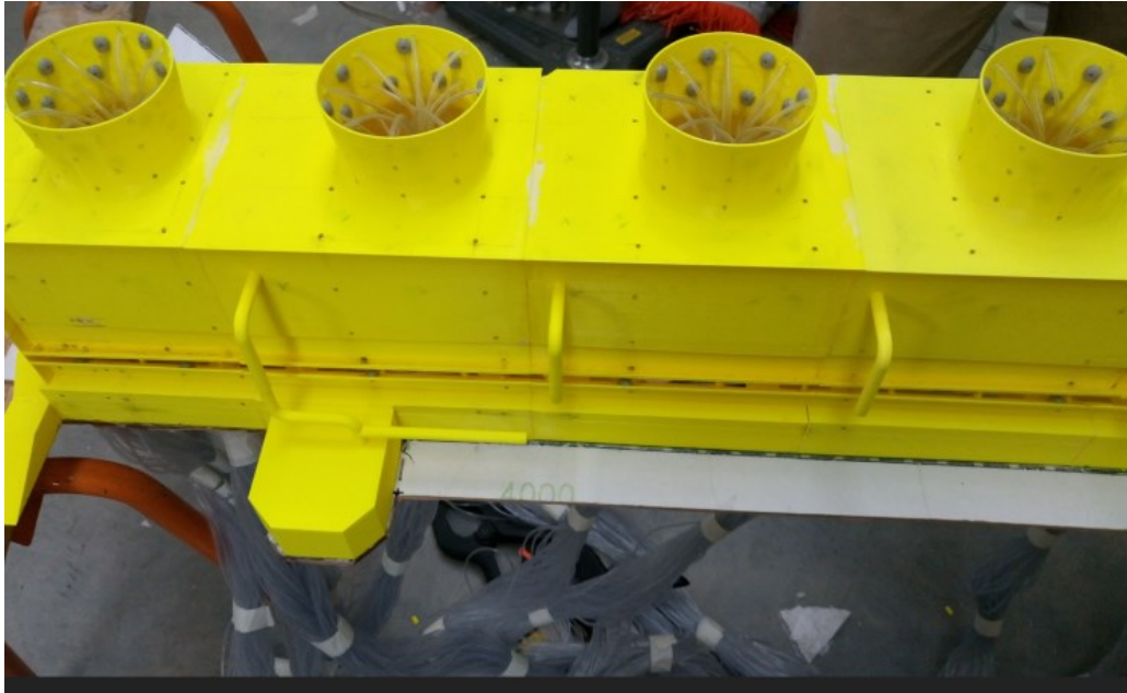
Figure 8: The study models were fitted with individual pressure sensors spread across the facades of the cooling towers and wind fences.
