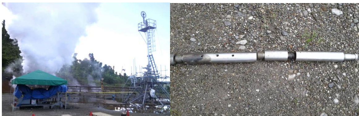
Figure 7 (Left Picture) Winch with the CTU set-up covered in tarpaulin to protect from inherent corrosiveness of geothermal fluids (left) and the well head set-up installed with the recovery spool for the injector head (right). (Right Picture) Injector head after the FMS test.
