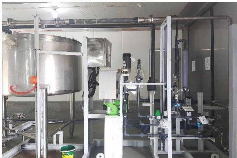
Figure 5: Stainless steel holding tank (left) and Pulsafeeder GLM series transfer pumps (right)
