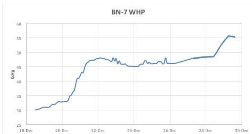
Figure 15: Well Head Pressure (WHP) of BN7 seen rising as it reacts to BN6 discharge
