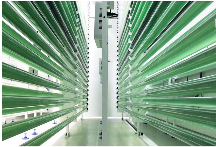
Figure 3: Photograph of the tubular photobioreactor at Blue Lagoon R&D center, used in this study.
