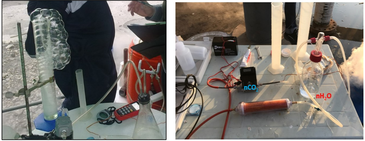
Figure 2: CO 2 -steam ratio measurement methods and related equipment, a) bubbling method and b) Flowmeter method.
