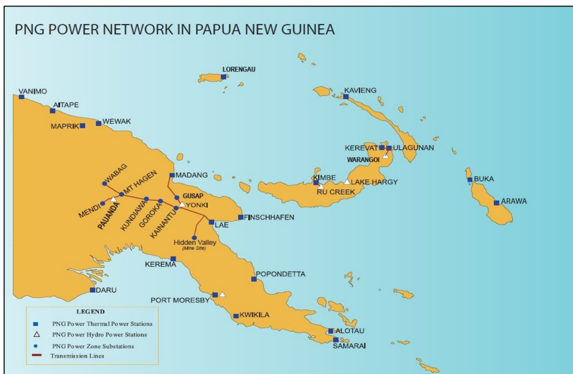
Figure 7: Map showing the power network and transmission system operated under monopolistic utility, PNG Power Limited in Papua New Guinea. (Red line indicates the transmission line and blue box indicates the power station/substations/generators) (Source: PPL, 2015).
