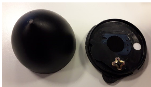
Figure 7: Solid state nuclear tracks detector used for Rn measurements.
