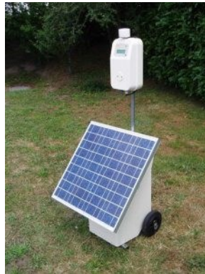
Figure 10: In situ alpha dosimeter for analysis of radioactive particles in the atmospheric dust.
