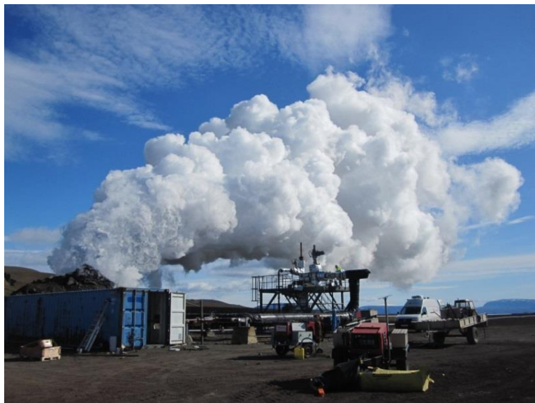
Figure 3. The flow of the IDDP-01 into a rock muffler produced dry superheated steam with only 0.1-0.2% of non-condensable gases. Initially corrosion products gave the steam a dark color but after a few minutes it became clear and transparent. The condensate had a pH 2.5-3 due to its HCl content. However experiments on wet scrubbing to remove acid gases from the dry steam were very successful (Hauksson et al., 2014). (Photograph courtesy of Kristján Einarsson).
