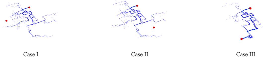
Figure 3. Effect of well positioning: Flow path for cases I, II and III with a well spacing of 800 m.
