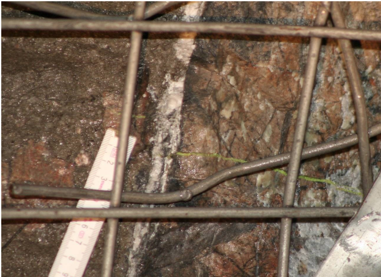
Figure 11: A photograph of a green-plastic propped hydraulic fracture crossing a calcite and quartz vein and leaving behind an offset. The scale is in millimeters and centimeters (after Jeffrey et al., 2009a).
