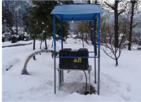
Figure 4: Onsite measurement of TC, TD and VHC of the 102 m deep geological formation.
