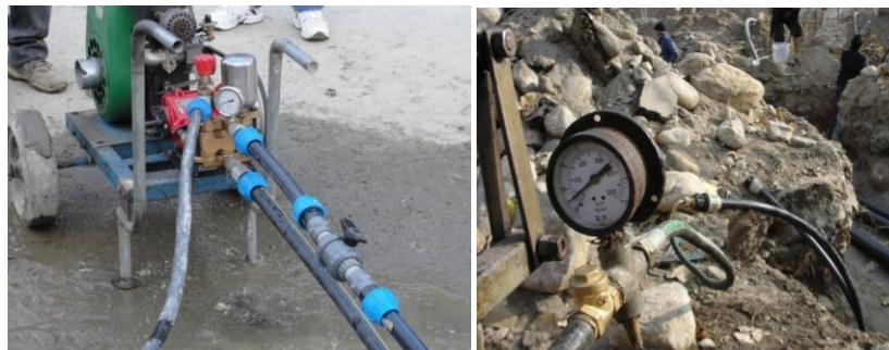
Figure 11: Pressure and leak testing of the ground loop, using (a) motorized pressure pump (150 bar), (b) manual Pressure pump (50 bar).
