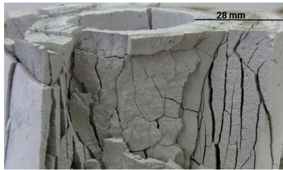
Figure 4: Oven dried grout specimen of a cement-sand-mixture (water/solid substance ratio 0.82) frozen and thawed out radially in the developed testing device (Anbergen et al., 2014a). The vertical cracks increased the axial hydraulic conductivity.
