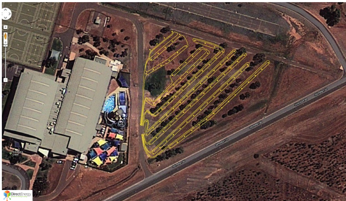
Figure 4: Vertical GHX design option (105 x 78m bores).
