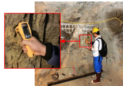
Photo 3: Measurement of rock surface temperature using an infrared thermometer
