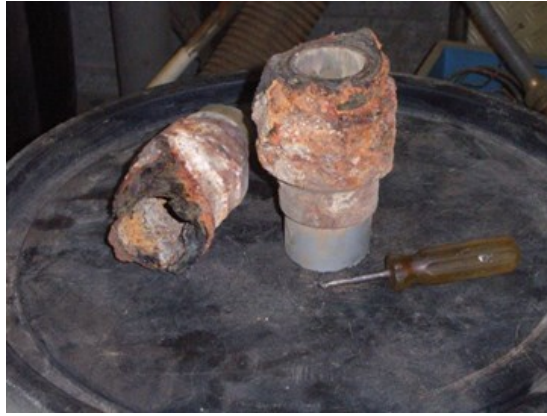
Figure 4. Corroded joints from the distribution system in the eating system in Öxarfjörður.
