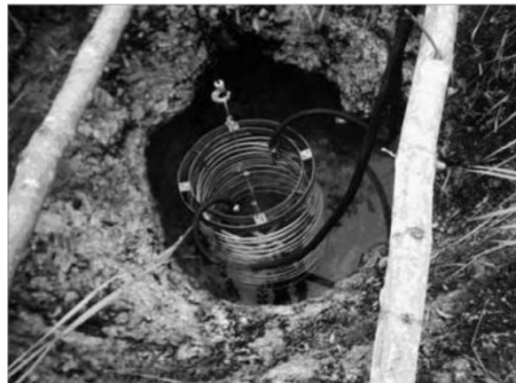
Figure 4: Downhole heat exchanger in natural geothermal well (Surana et al, 2010)
