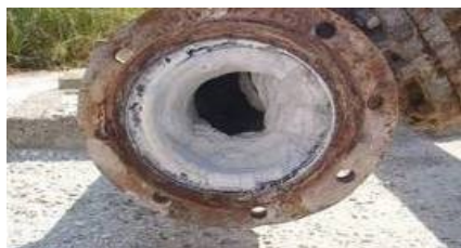
Figure 3a: Calcite scaling in Kizildere (Turkey) production wells in 2008
