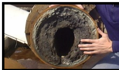
Figure 3b: Silica scaling in reinjection lines Iceland (Turkey)
