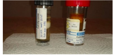
Figure 5b: Bacteria grow in cooling tower
