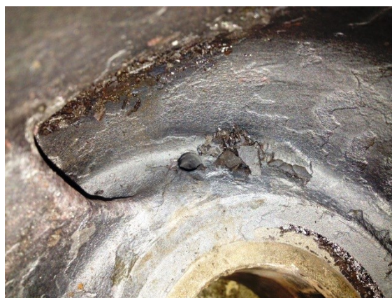
Figure 9: Metastibnite deposition on a pump impeller.
