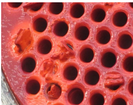
Figure 21: Softer, gel-like, deposits after dosing 30ppm of polymer
