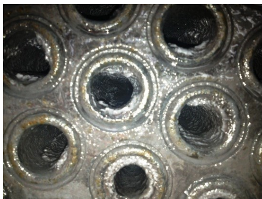
Figure 10: Soft paste-like deposit after dosing 4ppm.
