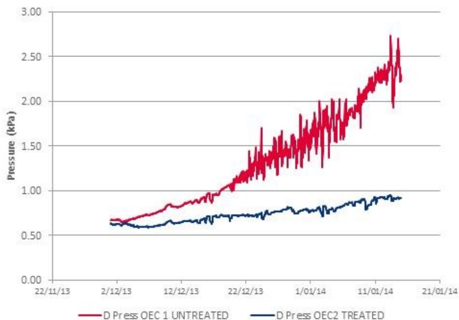
Figure 8: Differential pressures across two OEC units, one treated and the other not treated.
