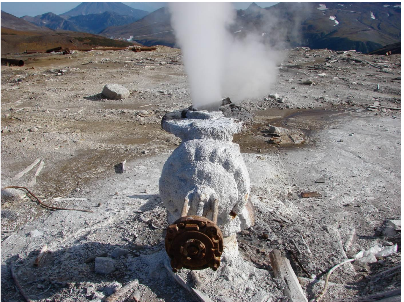
Figure 6: Aggregates of amorphous \text{SiO}_2 are precipitated from steam ( T\ 237^{\circ}\text{C} ).
