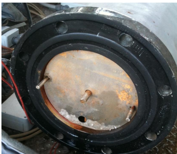
Figure 10: HUV Internal Baffle Outlet after Test 7
